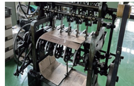
Figure 8. Jacquard card lacing machine (photo by author, 2021).
