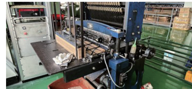
Figure 7. Jacquard card punching machine (photo by author, 2021).
